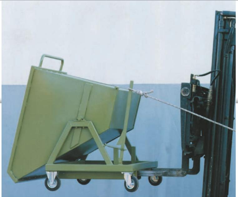
Swinging bucket with frontal emptying fitted with swiveling wheels to facilitate displacement. Upon request it can be supplied water-proof with coolant discharge tap.
